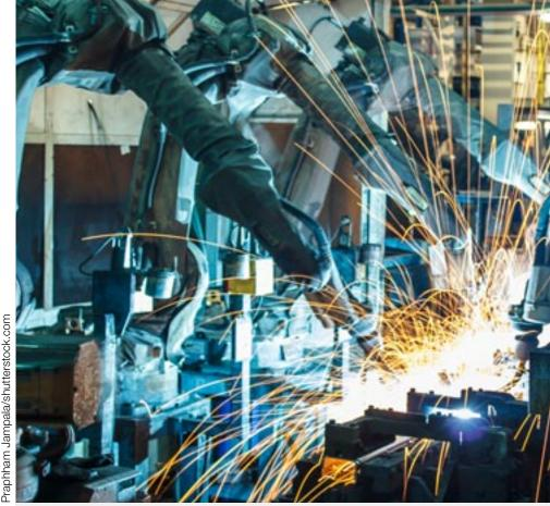
Welding robots on an automotive industry production line.
